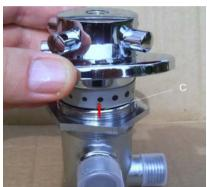
3 Lift off head and backplate and place safely to one side. Mark position of backstop band (E) to the valve cartridge as indicated in (D). Remove backstop and place aside. Protect cartridge head with appropriate size plastic bag and secure over carteidge head and valve body threads with masking tape to prevent plaster / debis contamination etc.
